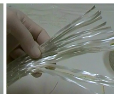
Step 3: Unravel the ends of the connector
