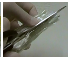
Step 2: Cut at the end of polypropylene weft
