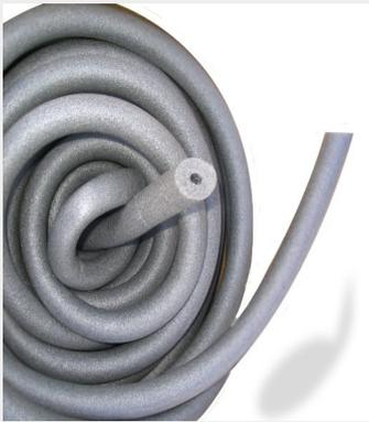
*Closed cell profile used to pre-fill joints or cracks to be sealed*
