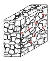
the connectors adjacent to each other by overlapping the strands inherent in the joints of mortar. Overlap should be of 20 cm at least.
