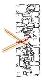
the substrate, and the injection of a suitable grout to restore the material continuity of the masonry.
