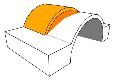
as an adhesive bridge with a consumption of about 0.7 Kg/  $\mbox{m}^{2}.$
