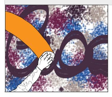
consumption rate indicated in the Technical Data Sheet. Once the anti-graffiti protection has been applied, it will be possible to remove any future stain with a simple jet of hot (80 ° C) pressurized (60-80 bar) water.
